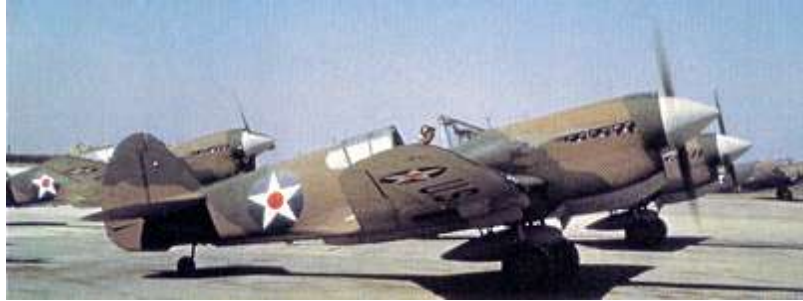
Left: Curtiss P-40C. The C model, powered by a 1040 HP Allyson, had a small air scoop a bit far back under the nose. It also had two .50 caliber machine guns on the nose and four .30 caliber on the wings. Right: P-40E. The E model had a larger air scoop closer to the nose and was powered by an 1150 HP Allison. It did not have nose guns, but carried six .50 caliber machine guns on the wings.
