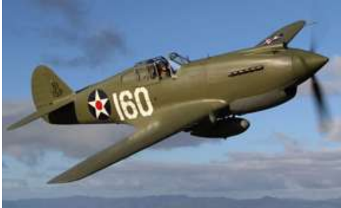
Left: Curtiss P-40C. The C model, powered by a 1040 HP Allyson, had a small air scoop a bit far back under the nose. It also had two .50 caliber machine guns on the nose and four .30 caliber on the wings. Right: P-40E. The E model had a larger air scoop closer to the nose and was powered by an 1150 HP Allison. It did not have nose guns, but carried six .50 caliber machine guns on the wings.
