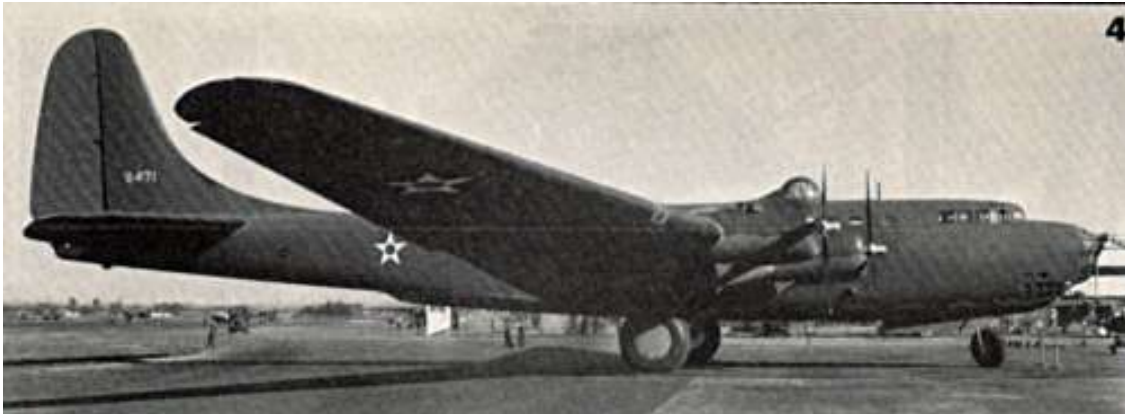
Douglas XB-19. Note advanced tricycle landing gear, but obsolete single tire on main landing gear which damaged runways on landings.
