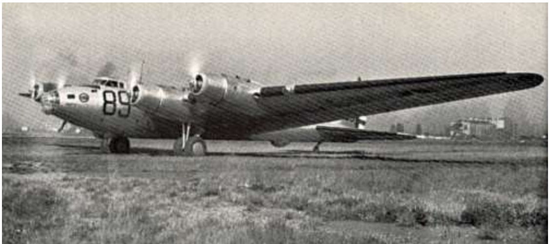
Boeing XB-15. In this case, the landing gear is the old fashioned tail wheel type, but they have distributed the weight of the plane on double-wheel main landing gear.
