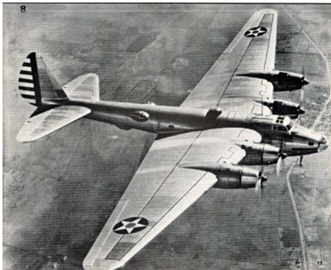
Left: The Boeing XB-15. Note the tremendous size of the wings in relation to the fuselage. This same wing design would later lift the Boeing 314 Clipper flying boats. Right: The Douglas XB-19.
