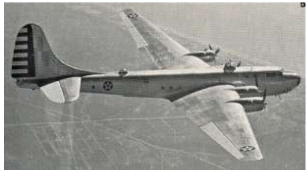
Left: The Boeing XB-15. Note the tremendous size of the wings in relation to the fuselage. This same wing design would later lift the Boeing 314 Clipper flying boats. Right: The Douglas XB-19.
